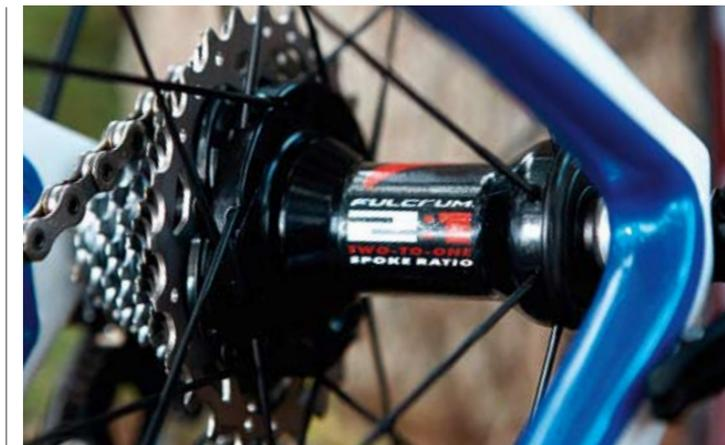
▲ The rear Fulcrum wheel uses 16 spokes on the drive side to eight on the non-drive side for power transfer
